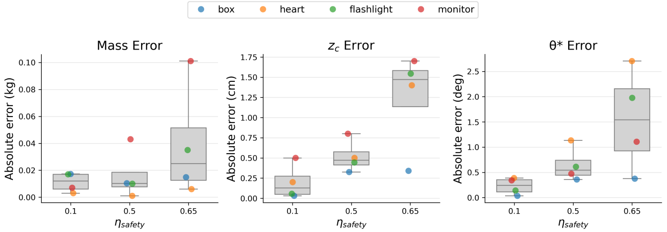
Fig. 6. Absolute error in mass, CoM height, and toppling angle for all tested objects as a function of the safety margin parameter \eta_{\text{safety}} . Each box plot aggregates results from each of the four objects for a particular safety margin. Errors increase with conservative safety settings due to reduced observability near the toppling threshold, though performance remains within acceptable bounds for practical manipulation.
