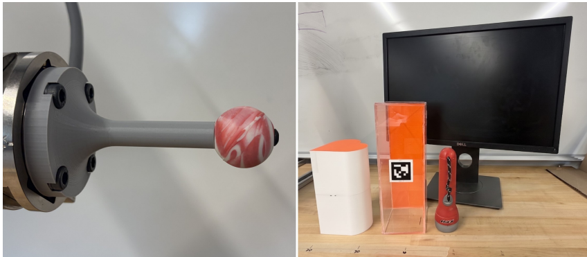
Fig. 5: (left) Robot finger used for both interaction modes. High-friction spherical tip provides better traction during press-and-pull and reduces required press force magnitude. (right) four objects tested, varying in size, shape, weight, friction, and CoM.
